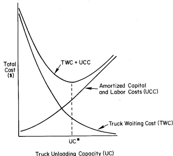
FIGURE 2. SCHEMATIC REPRESENTATION OF TRUCK UNLOADING SYSTEM
