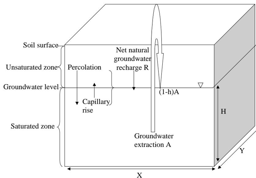
Fig. 1. Schematic representation of the water flows in the unsaturated and saturated zone. The subsoil consists of an open layer on top of an aquifer, which means that the hydraulic resistance of the top layer is low.
