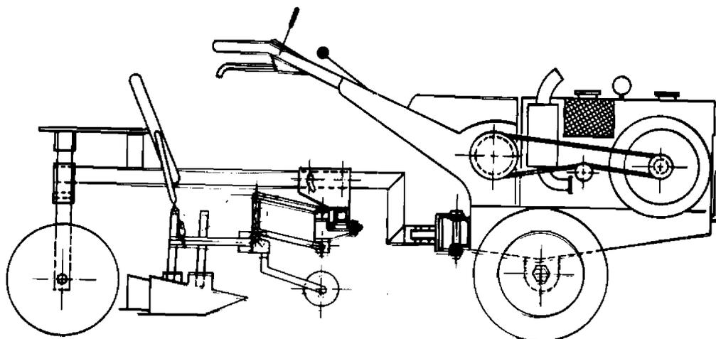
Fig.2. Multi-purpose toolbar with seat and wheels fixed to a two-wheeled tractor (After Rhebergen, 1976)
